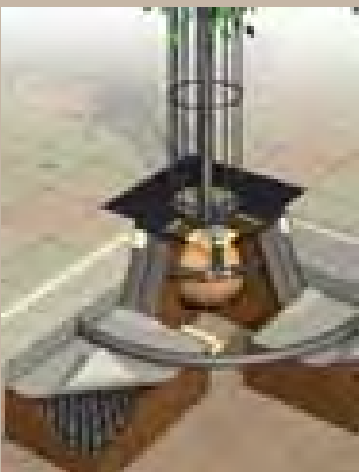
The use of root barriers and root cells prevents damage to surface materials and service ducts
