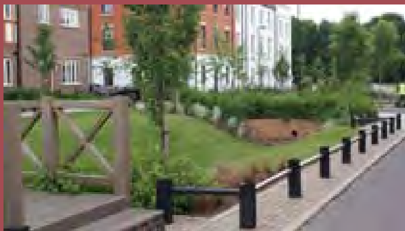
Swales as a means of rainwater infiltration can form an integral part of the landscaping; an early consideration in new landscaping schemes ensures functional as well as visual qualities
