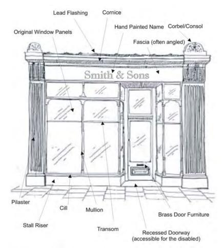
**Figure 6.1**: Elements of a traditional shop front, comprising pilasters (or columns), traditionally topped by console boxes and a fascia (often angled), a recessed doorway, and display windows (often divided with vertical mullions and horizontal transoms) sitting above a rendered or tiled stallriser (minimum 450mm in height).
