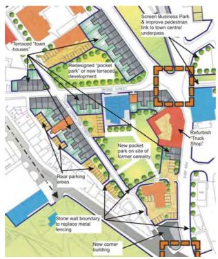
**Figure 8.3:** Indicative masterplan layout for new development on the Lower Coronation Street/Bridge Street/Iron Row area. Similar to the proposals for Upper Salisbury Street, the development of terraced "town houses" could re-establish the original plot building lines. Where new development cannot be accommodated due to narrow plot widths etc... consideration should be paid to the provision of defining stone walls and planting. Such secondary streets should be designed as "home zones".
