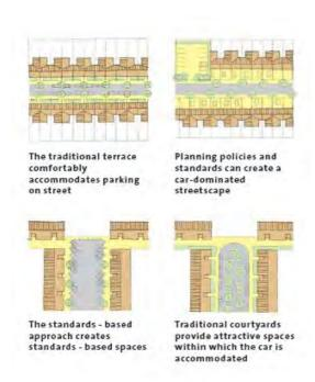
**Figure 5.5:** Examples of how on-street parking can be positively incorporated into streetscapes, rather than sticking to rigid "highway standards" which can create car-dominated spaces (*Source: "By Design", DETR*, 2000).
