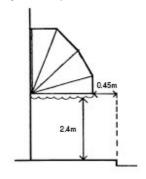
Figure 6.3: Dutch-style retractable "fan" blinds are not suitable, as they hide architectural details and interrupt building elevations.
