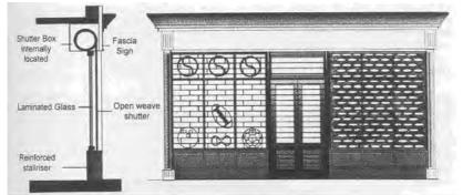
Figure 6.4: Left – Diagram showing an appropriate internally mounted shutter box; and Right - Illustrations of three types of acceptable internal "open weave" retractable shutters or grilles (Source: Mansfield Council's "Shop Front Security Design Guidance", 1994).
