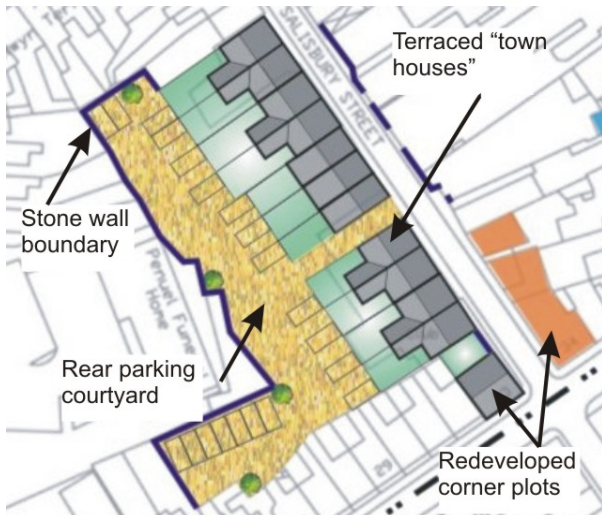
Figure 8.2: Indicative masterplan layout for new development on the Upper Salisbury Street Regeneration Site, showing how terraced “town house” development could re-establish the original building line, with parking accommodated within a rear courtyard, and the need for stone wall boundaries to define public/private spaces to the rear of Castle Street properties. The two buildings on the corner or Market Street/Upper Salisbury Street should also be redeveloped, retaining as much of the original buildings’ detailing as possible.
