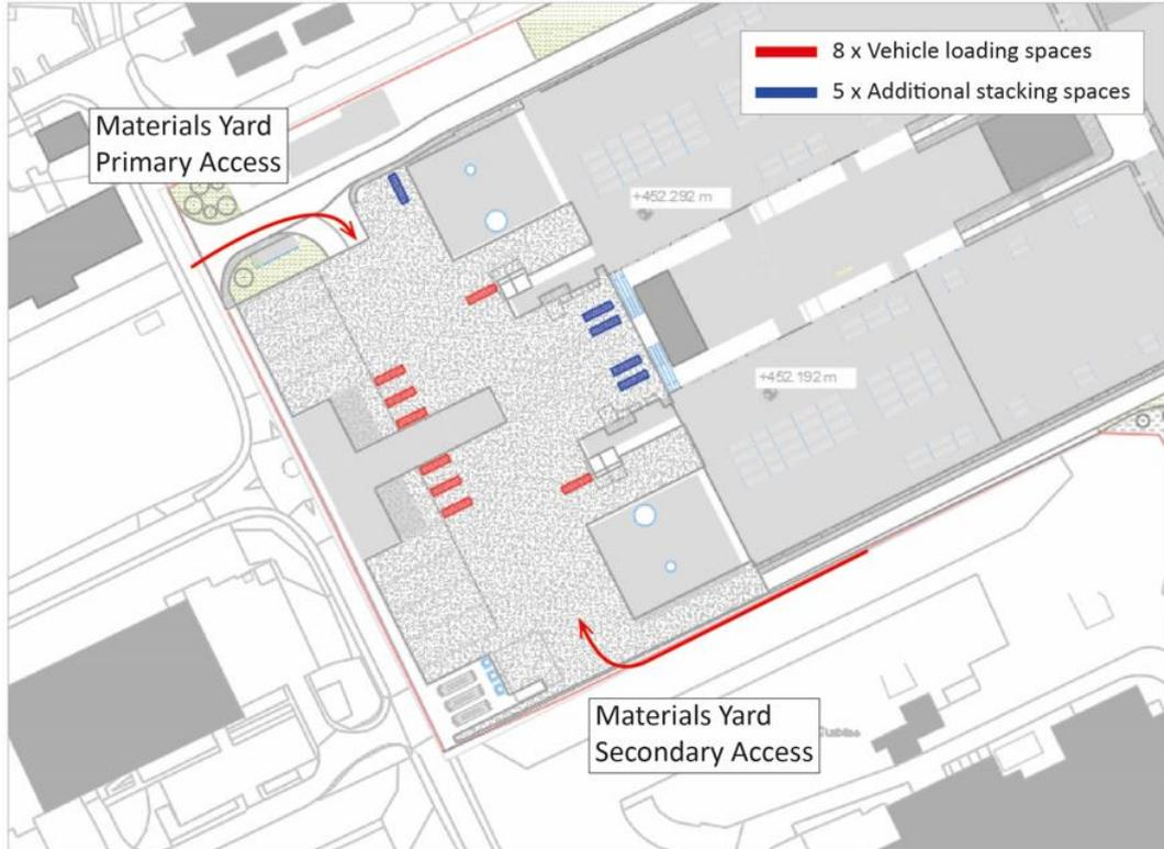
Figure 1: On-Site Stacking Space – Materials
