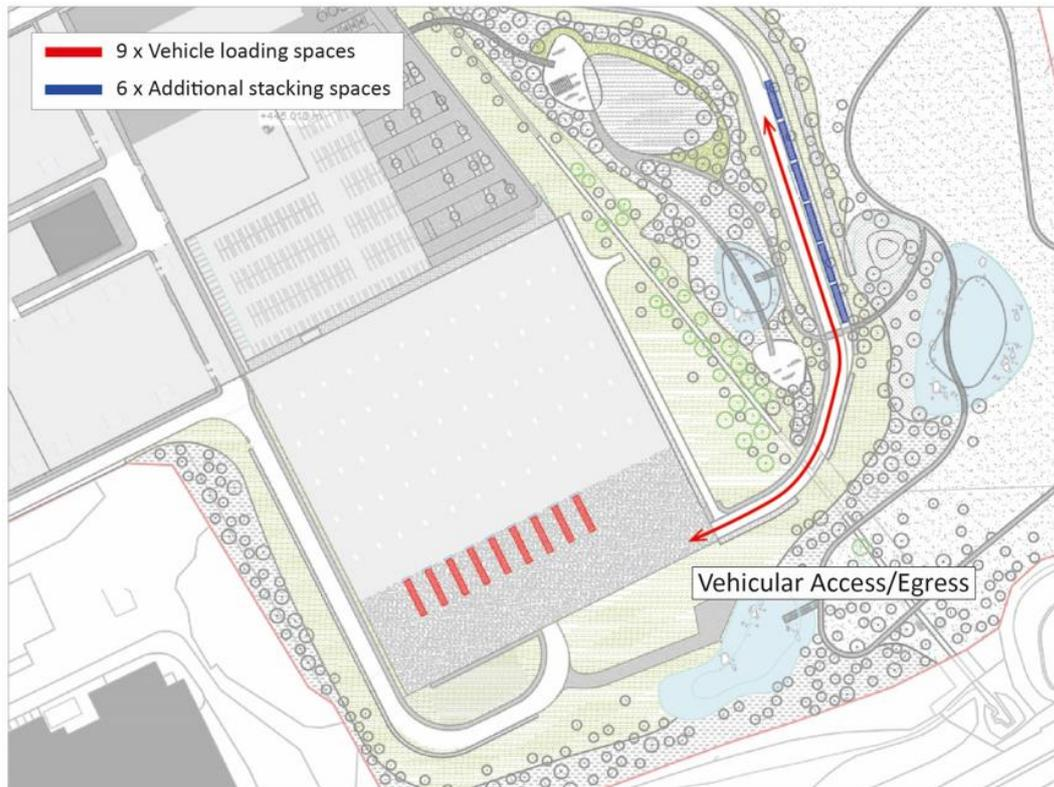
Figure 2: On-Site Stacking Space – Glass Transportation
